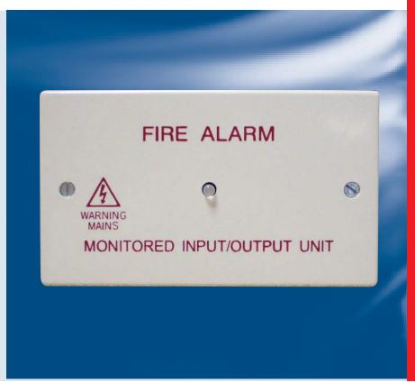
The Protec 6000 series MICCO is a loop powered fault monitored input and a volt free clean contact output interface. An on board isolator is provided which protects against loop short circuits on either the incoming or outgoing loop connections.
